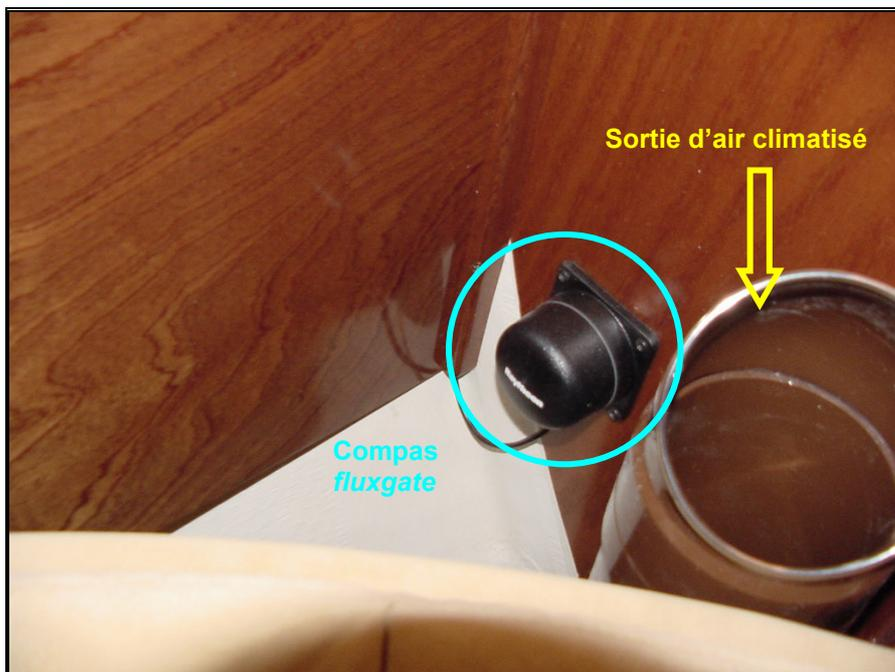
Figure 98 – Compas fluxgate
